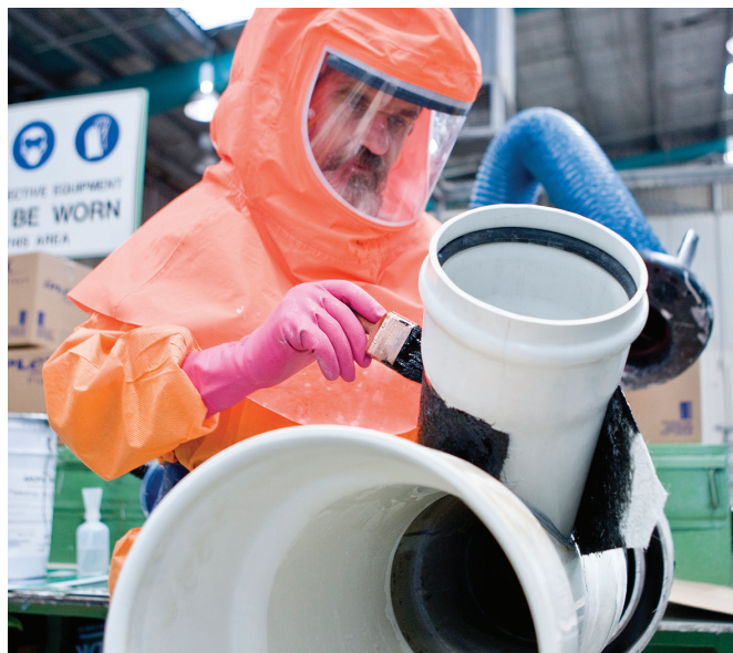
BlackMax PVC Junction in manufacture
