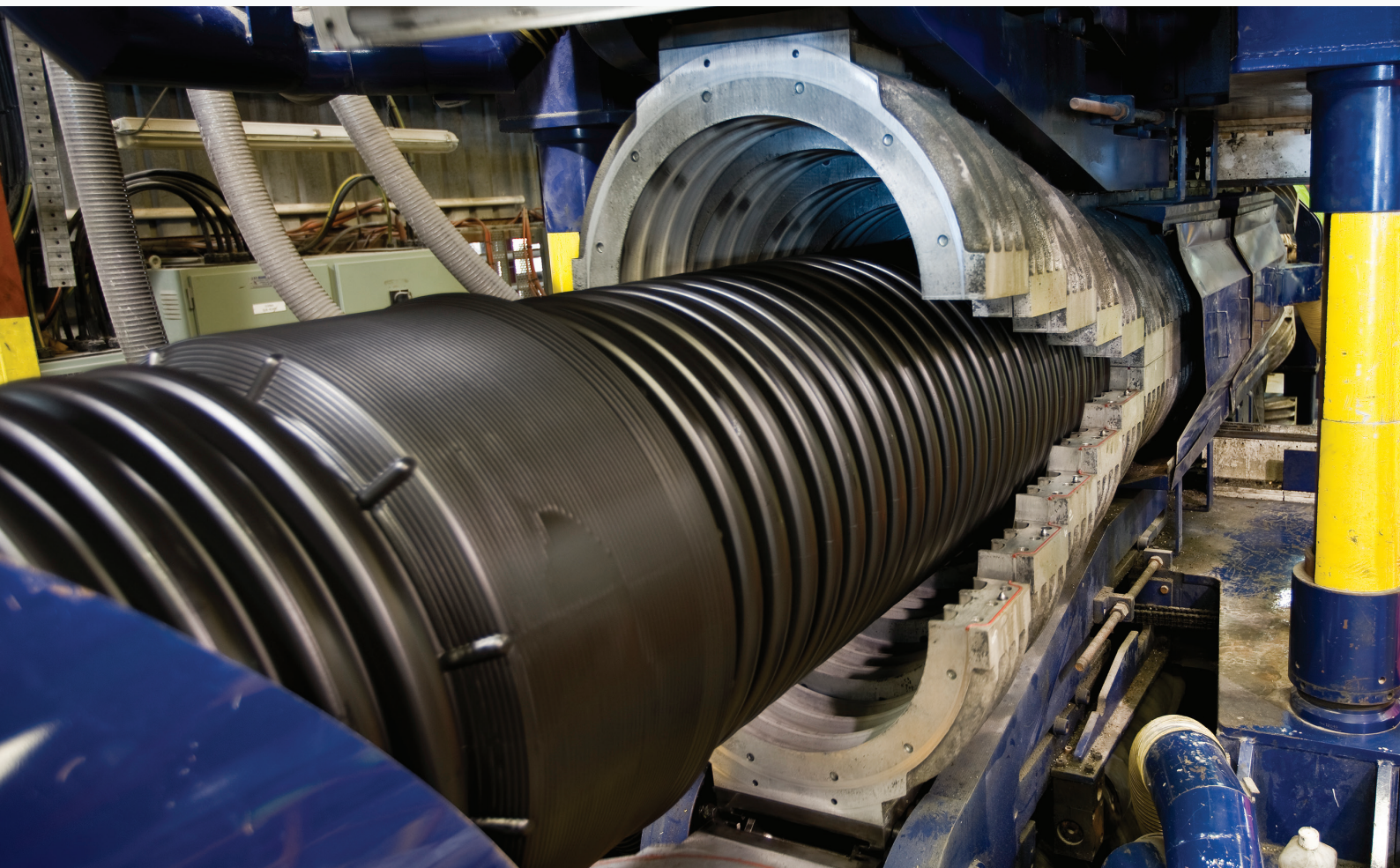
BlackMax pipe manufacturing process
