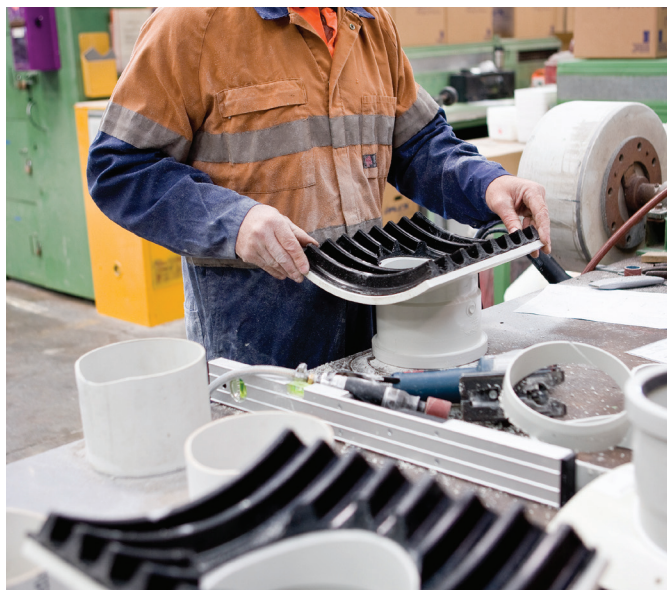
BlackMax PVC Saddle in manufacture
