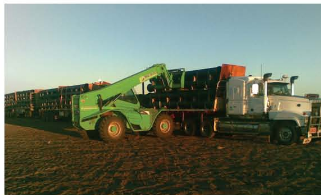
Irontite® pipes are safely unloaded with approved lifting equipment at Cloncurry, Queensland
