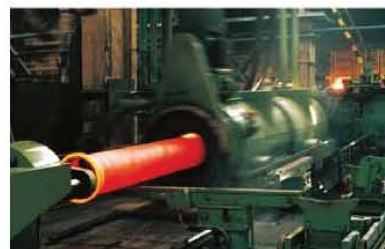
Irontite® ductile iron pipe centrifugally cast in machine with water cooled steel moulds
