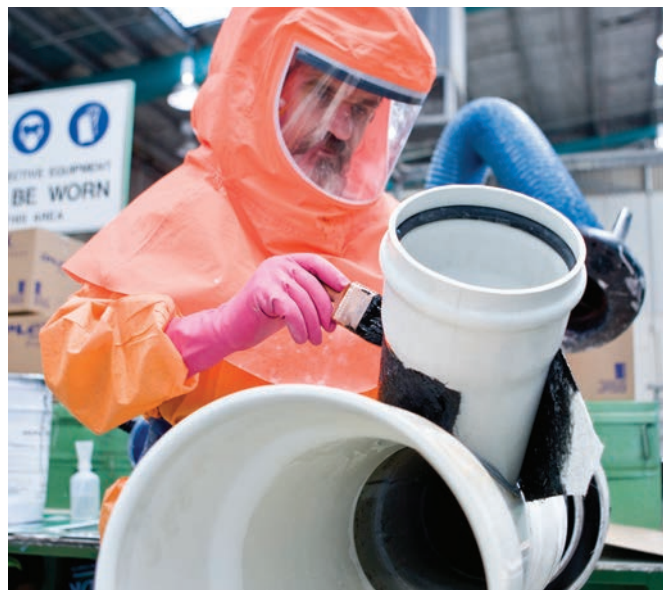
BlackMax PVC Junction in manufacture
