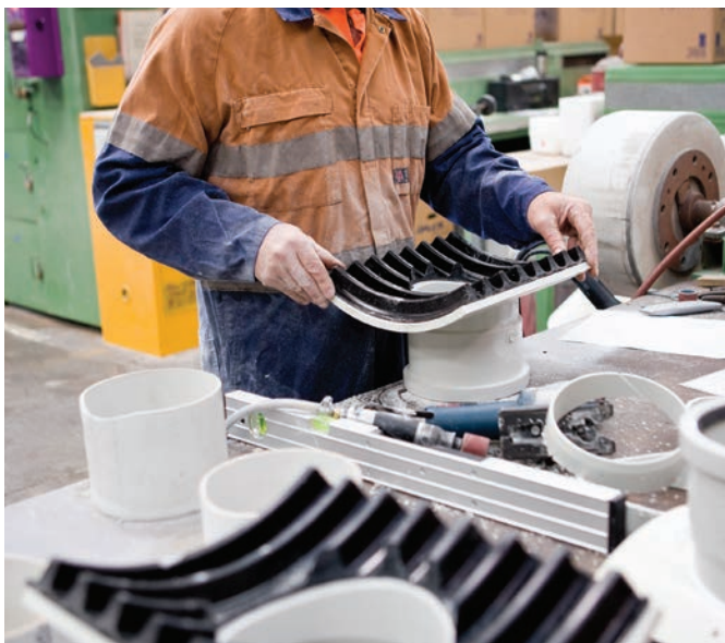
BlackMax PVC Saddle in manufacture
